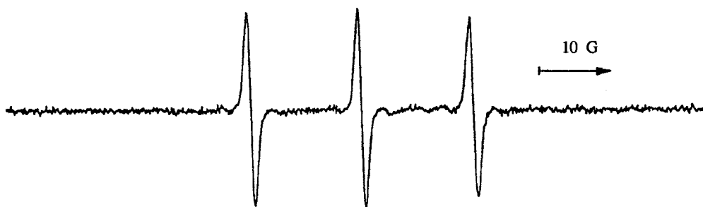
Fig. 1. EPR spectrum of 0.1 M M_3PO solution in water using the best purified sample of M_3PO available; instrument settings for ESP-300E Bruker EPR spectrometer: modulation amplitude 0.975 G, microwave power 20 mW, scan time 83.9 s, sweep width 100 G; receiver gain: 1 \times 10^6 .
